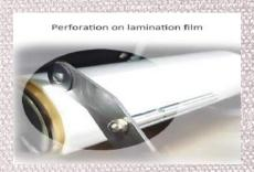
Auto perforating on side of lamination film, which makes easy to burst sheets.
