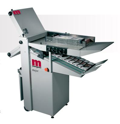
A powerful suction feed handles a wide range of coated or non-coated material and incorporates side lay alignment of the sheets before they enter the fold plates. The feed table also has a suction chamber to control curled or statically charged paper.
