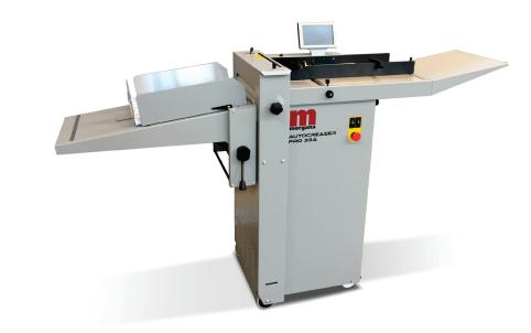
The AutoCreaser Pro 33A provides the complete solution to the problem of cracking that occurs when folding digitally printed output. It is equally effective in dealing with conventionally printed card, laminates or crossgrained stock.
